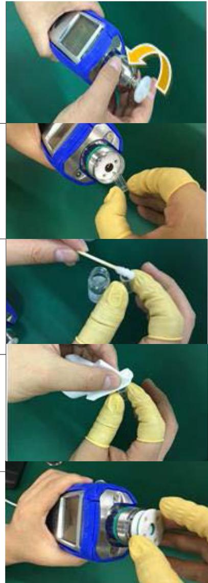
***Always re-calibrate the PID after cleaning the lamp and/or sensor.***
