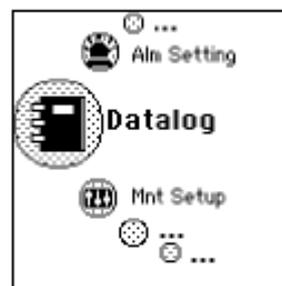
In the datalog submenu, you can adjust the interval and clear all logged data.
